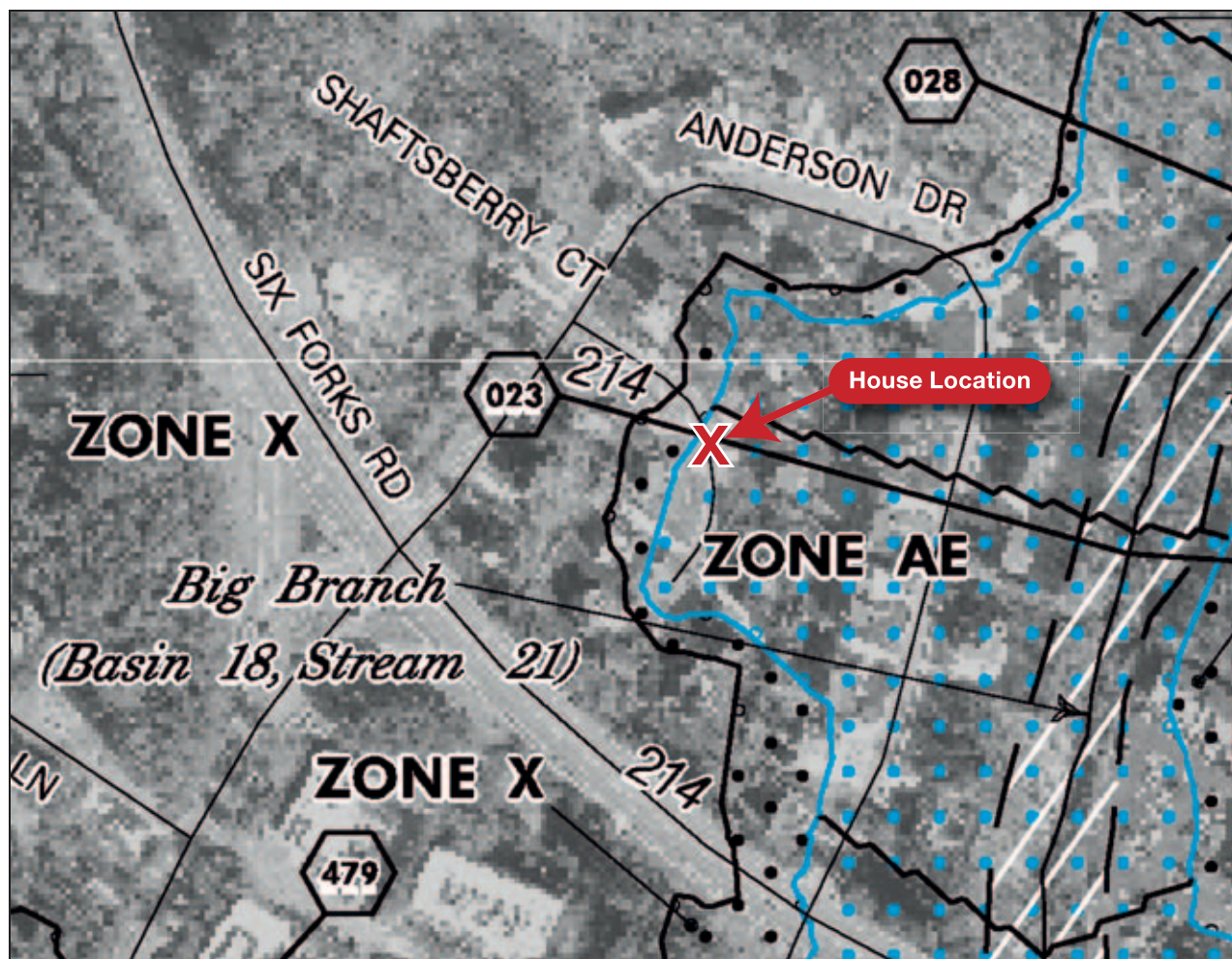
Figure 4-2. House and stream location on the DFIRM
